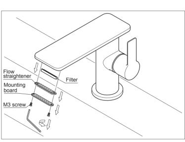
If the flow rate gradually decreases after some time, it usually results from poor water quality leading to blockage of the filter. Please clean the filter as shown in figure above: Turn off the handle, unscrew the M3 screw with the S2 spanner, take off the mounting board, the flow straightener and the filter in turn, wash the filter and then install them back.
